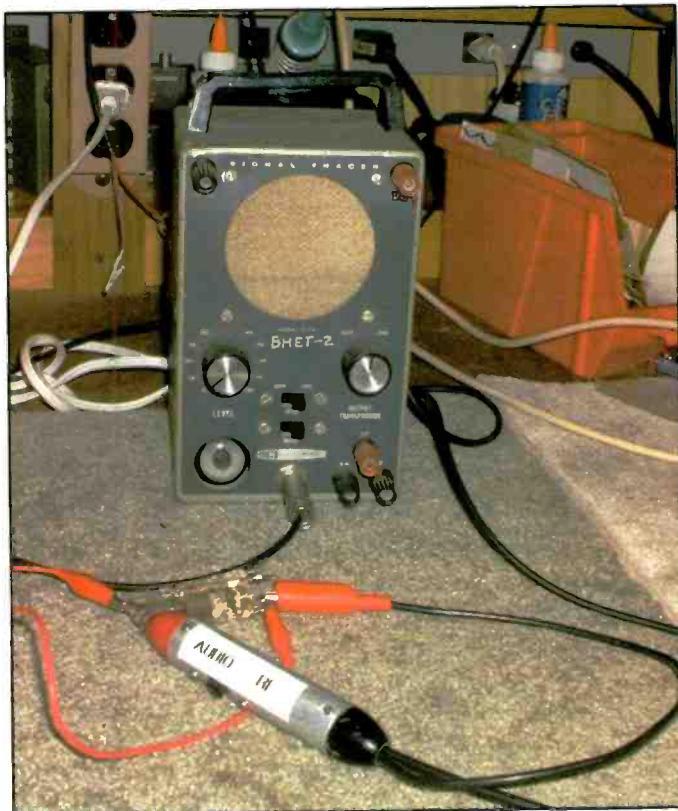
Photo C. The Heathkit IT-12 signal tracer features a noise test that applies a high DC voltage to the part under test. Any arcing or breakdown causes AC noise artifacts to ride on the DC level; they are then capacitor-coupled to the tracer's audio amplifier so they can be heard on the speaker. The test worked better than expected and proved the transformers were defective. Note that the probe leads are applied to both windings, not across the primary or secondary!
