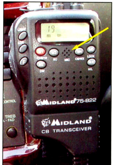
A close-up of the 75-822 with the microphone hole noted by the arrow.
