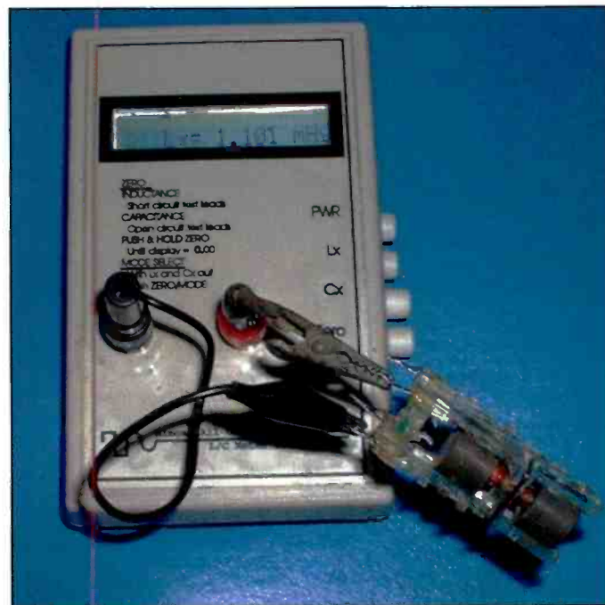
Photo G. The AADE L/C meter provides an accurate and quick means to determine the actual inductance value of the individual primary and secondary windings.
