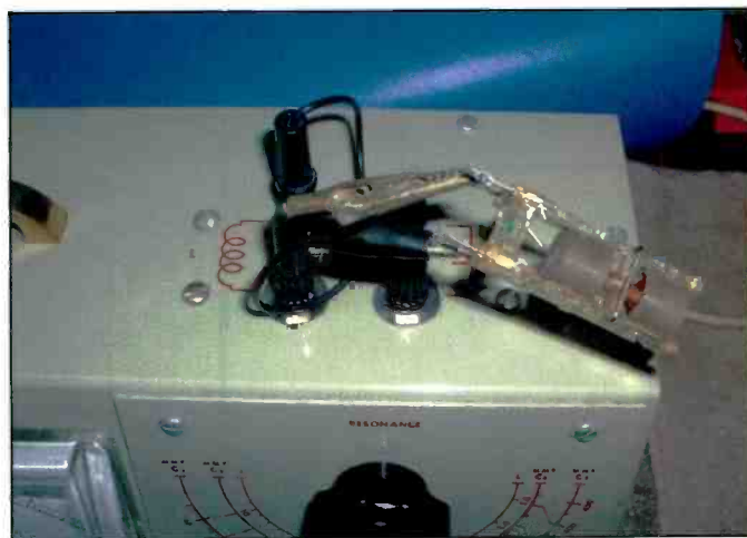
Photo I. The coil (or IF transformer winding in this case) connects with short leads directly to the coil test terminals on top of the QM-1 test instrument.
