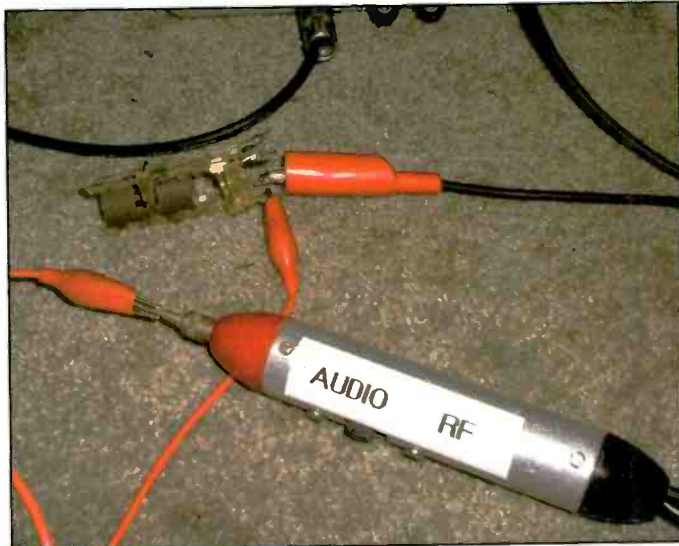
Photo D. Here's a close-up of the probe and hookup for the noise test. Note that the probe must be set for audio in order to pass the DC voltage to the part under test.
