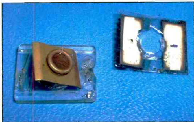
Photo F. In this photo I've gently heated the rivet and pushed it through the polystyrene material once it was softened enough to remove it. This permitted access to the silver mica capacitor wafer for removal. Note the square tensioning spring on the other side of the rivet, inside the transformer shell. These parts are discarded and not reused.
