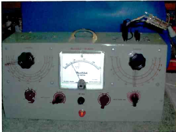
Photo H. The author's QM-1 Q meter is rather exotic and is seldom seen in service shops, but it proved its worth for determining the proper capacitor values needed to resonate each winding at 455 kHz.
