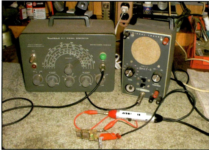
Photo J. The author's Heathkit SG-8 signal generator and IT-12 signal tracer indicate that the IF transformer can be tuned to resonance.
